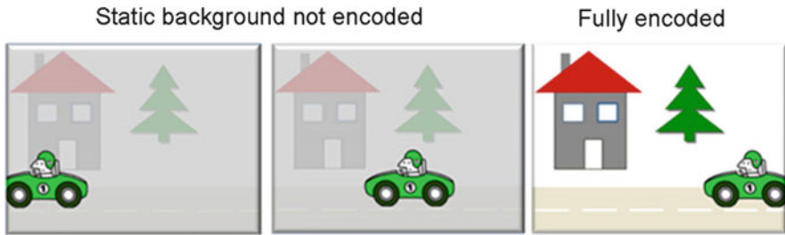
Fig. 6.2 Difference coding only codes the first image, shown here on the right . Subsequent images reference the first picture for the static elements, i.e. the house and tree. This static grey background is not transmitted. Thus, it is only necessary to code moving parts—the car—which vastly reduces the data that must be processed
